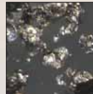
Crystalline graphite structure in oil 168x
